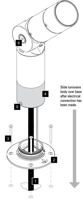
Surface Mount (Type A) For direct mounting to a flat surface
