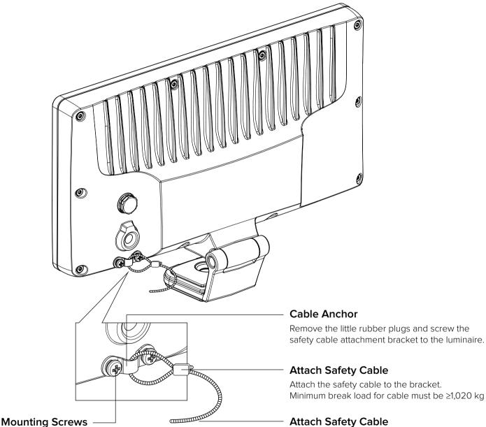
Be sure to use spring washers provided (between screw head and safety anchor) to ensure screws don't loosen over time.
