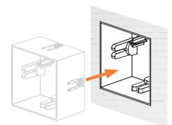
Align edge of the mounting kit with the surface of the wall and secure box in place.
