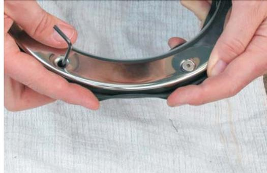
12. Place cover on fixture lining up allen-key with any hole
