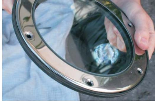
10. Insert 5 screws all the way into cover, leaving one hole without screw. Place allen-key in 6th cover hole
