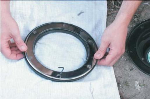
11. Ensure cover is inside the lip at the edge of the seal
