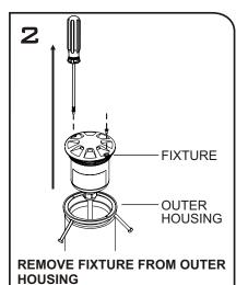
Remove the two screws fom the lid of the fixture. Carefully pry the fixture from the brass collar and place in a safe location for future installation
