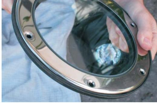
10. Insert 5 screws all the way into cover, leaving one hole without screw. Place allen-key in 6th cover hole
