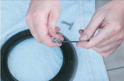
11. Insert 5 screws all the way into cover, leaving one hole without screw
