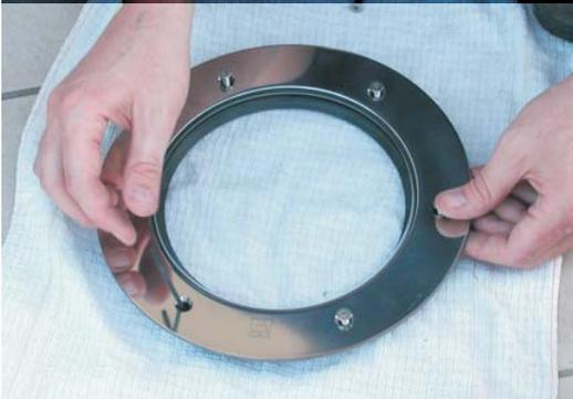
13. Place cover on fixture lining up allen-key with any hole
