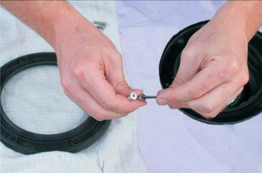
11. Insert 5 screws all the way into cover, leaving one hole without screw. Place allen-key in 6th cover hole
